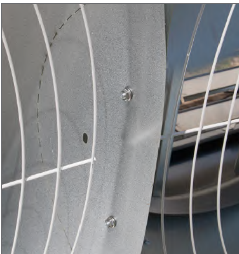
Galvanized metal cone features perforated edges that allow fans to be installed closer to each other in retrofit applications, reducing the need to reframe each fan opening.
